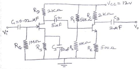
Given:  $V_{GS} = -1V$ ,  $I_{DSS} = 8mA$ ,  $V_P = -4V$  for JFET and  $h_{ie} = 1k\Omega$ ,  $h_{fe} = 100$ ,  $V_{BE} = 0.6V$  for BJT.
